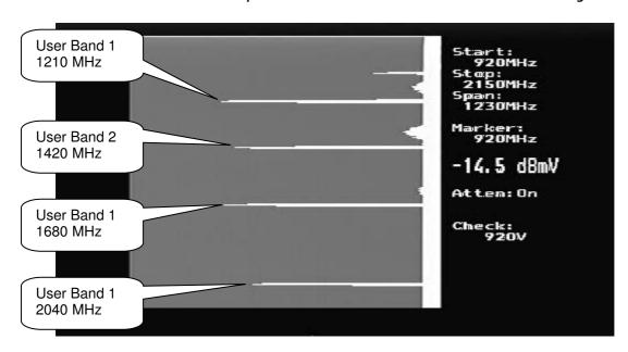
At the end of the test, the results of measuring the User Bands are presented.
