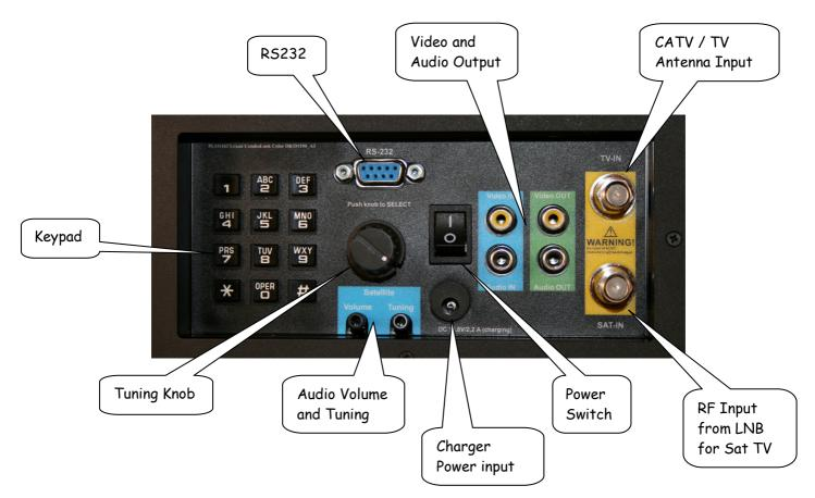
**Power Switch)** On battery power, this turns the instrument on and off. When the charger is connected, the instrument will charge with the switch off, and operate when on. The instrument will not charge when operating.
