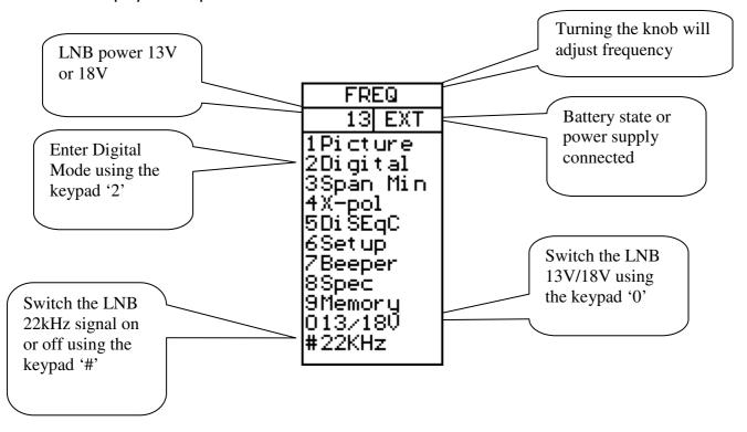
When the operation can use a memory location, the lower portion of the LCD shows the current memory selection. For this case, the knob is used to change the memory position number that the 'Save' will use.
