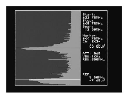
This measurement can also be made from Spectrum samples saved in memory. After a spectrum is loaded from memory with "Memory -> Load" choose" Ref mrkr" and use the knob and set the first marker position with "Ref set" and then use the knob to define the second reference marker.
