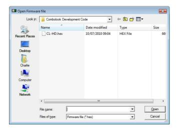
Normally, the firmware will be in the same direction as "FDLDVB.exe" but if not, you can navigate to the correct directory and select the firmware file. Once the file is selected, the firmware loading will take about 10 minutes and then the Firmware Downloader program will display "Download Complete".
