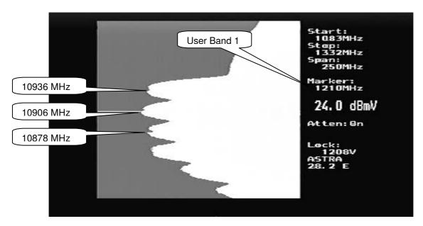
The UniCable test (Spec -> UniCable -> Uni Test) allows full testing of a UniCable LNB. This test takes about 20 seconds to check each User Band. During the test, the four User Bands are identified and any offset found is used for further UniCable tuning.
