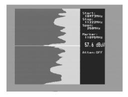
Rotate the LNB so that either the Horisontal or Vertical polarisation will be in its max-position –adjusting the **cross-polarisation**. Pressing the nr 3 button again (span Max), gets You back to "Max zoom out".
