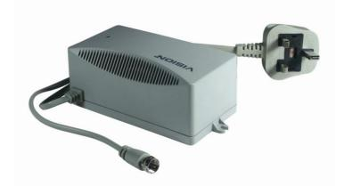
V5 and V9 IRS can be powered using the V5-024 via the H,Lo and H,Hi trunk cables or by DC connection into the auxiliary DC socket of a multiswitch. This flexibility means that power can be inserted at almost any point in the system even where there is no main power near the headend amplifiers.
